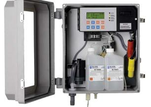
This in-line analyzer allows for the simultaneous monitoring of both pH and chlorine. The analyzer has two 4-20 mA outputs so both parameters can be configured with most SCADA systems. The analyzer follows the EPA's recommended DPD 330.5 method for Chlorine determination. By combining pH and Chlorine, the analyzer reduces cost, wall space and the need to maintain two separate controllers.
